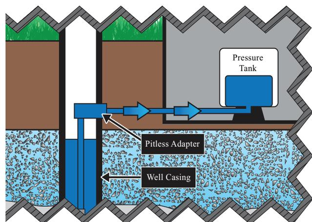
Figure 1. Water is pumped from the well through the pitless adapter to the pressure tank, then to various water fixtures in the building.
