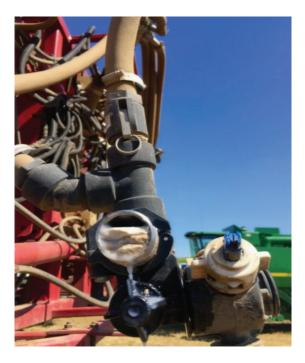
Fig. 2. Pesticide residue accumulation at an end cap.
