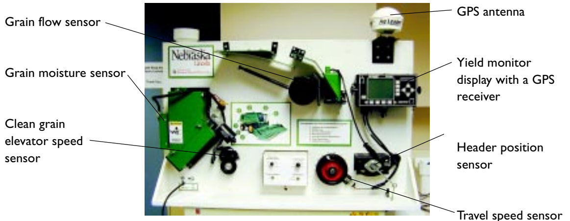
Figure 1. Teaching display with the major components of a grain yield mapping system.
