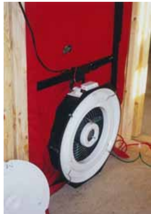
Figure 4. A blower door test can determine how airtight a home is.
