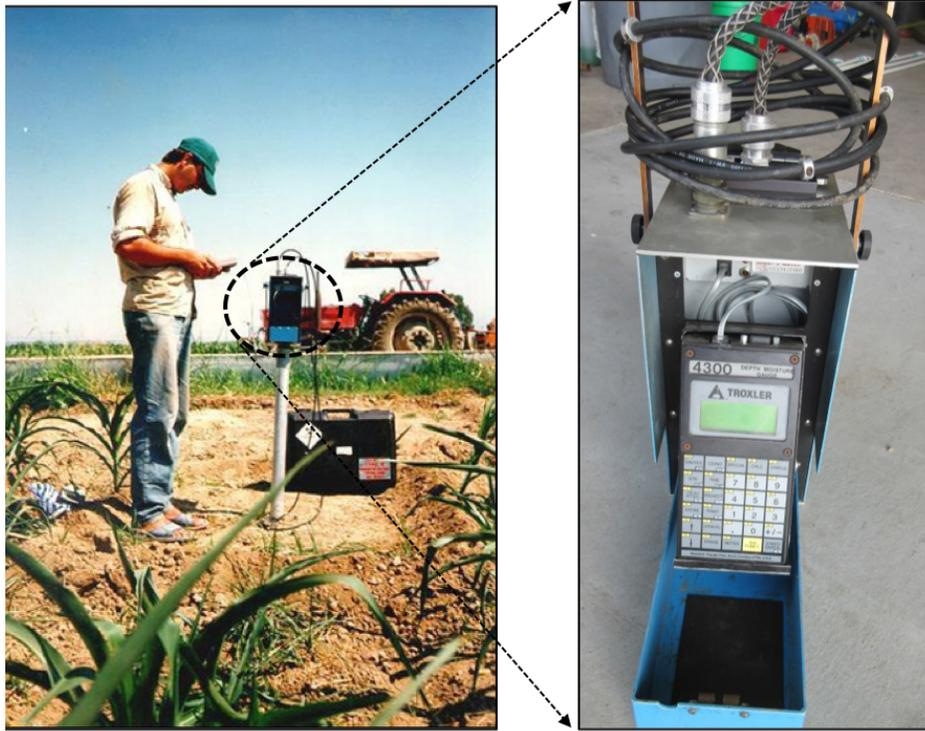
Figure 3. Taking standard counts using a Troxler 4300 neutron probe (Troxler Electronic Laboratories Inc., Research Triangle Park, North Carolina) that is attached to an aluminum access tube in approximately 50% clay soil.
