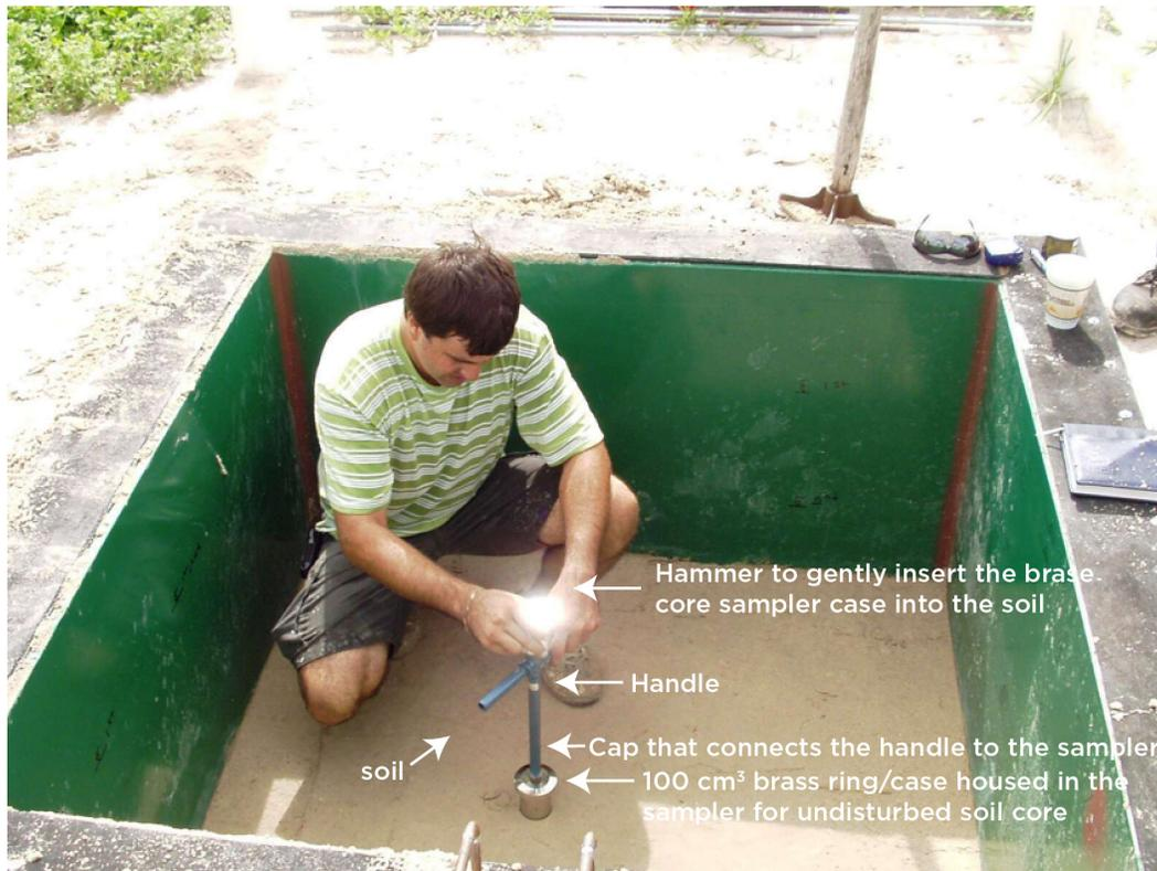
Figure 2. Taking soil bulk density samples in a weighing lysimeter using an undisturbed soil core sampler. (100 cm<sup>3</sup> = 6 in<sup>3</sup>)
