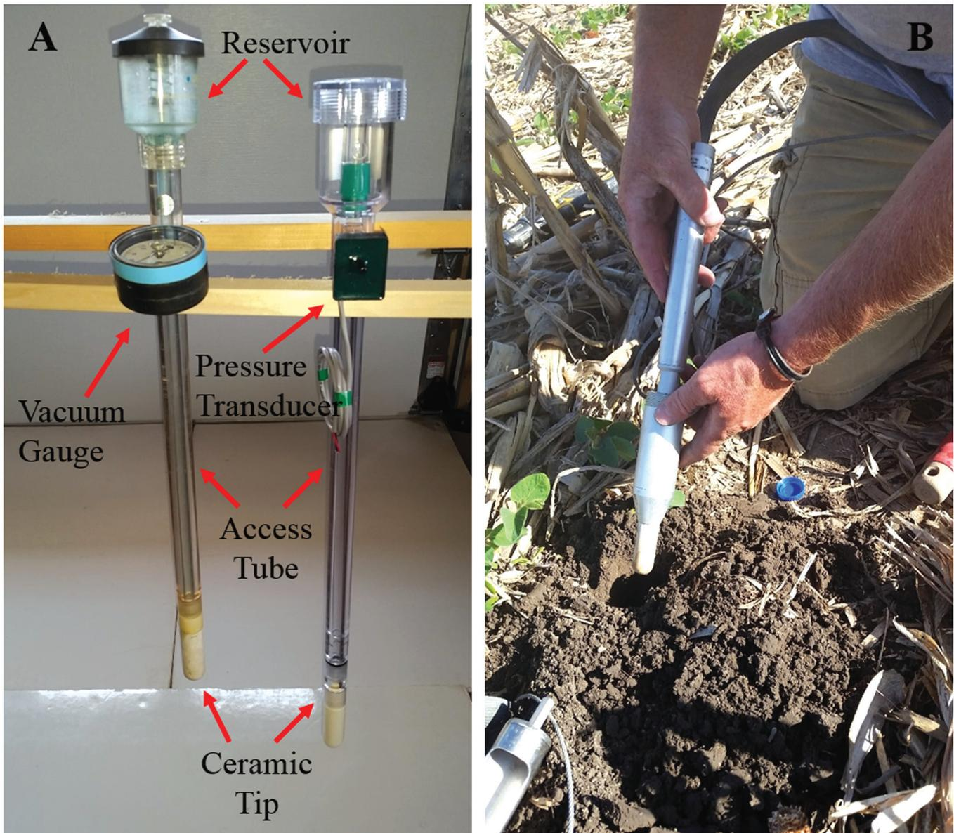
Figure 5. Two traditional tensiometers, one with a vacuum gauge (Soil Moisture Equipment Corp., Santa Barbara, CA) and the second with a pressure transducer (Irrometer Co., Inc., Riverside, CA) (A), and a tensiometer developed by Hortau, San Luis Obispo, CA) (B).
