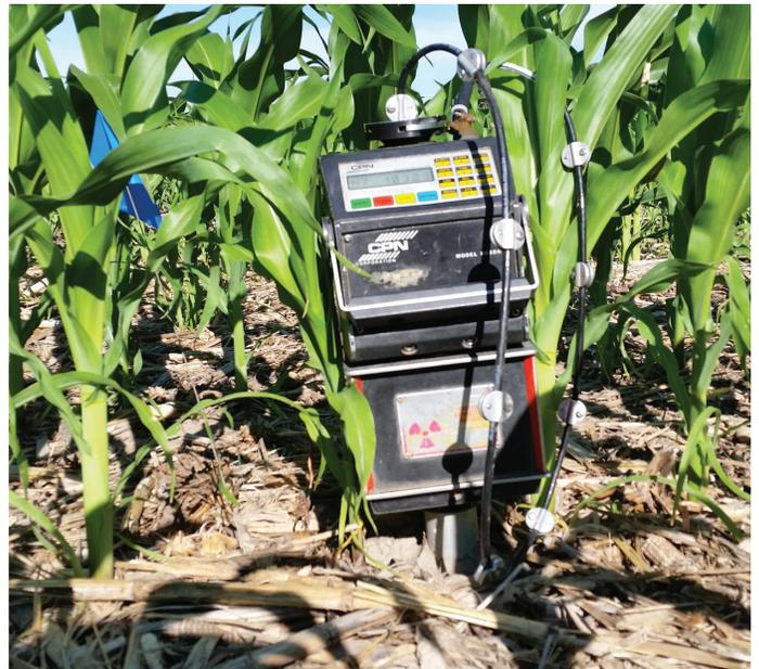
Figure 2. Installation of an access tube (A), standard count measurement (B), and in-season field measurement of a CPN 503DR Hydroprobe™ (neutron gauge) (C).
