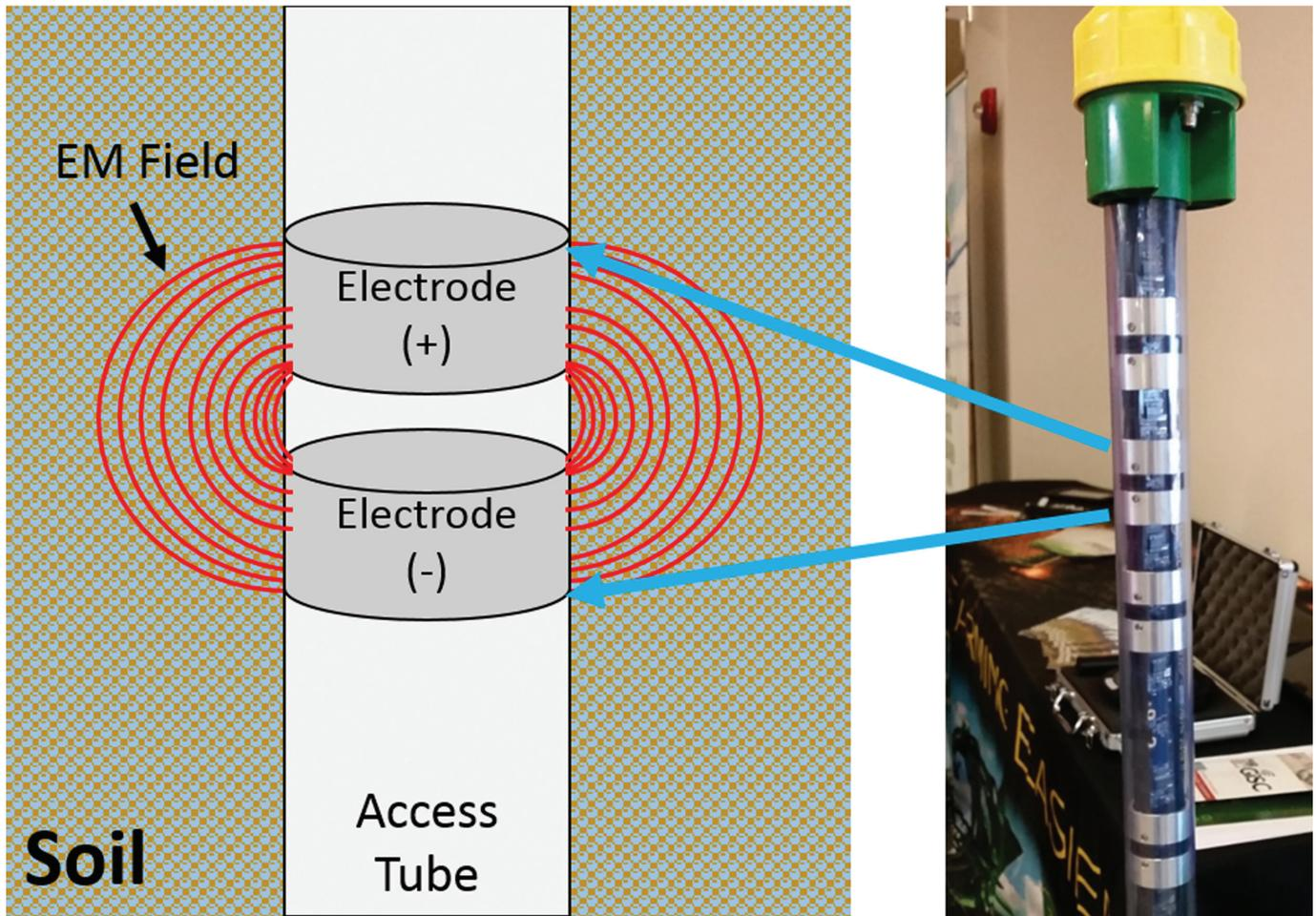
Figure 3. Capacitors located within a John Deere Field Connect™ capacitance probe with an illustration of a capacitor's electromagnetic (EM) field penetrating the soil.
