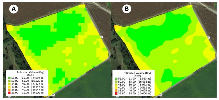
Figure 4: Grid-based (50 ft square) yield map (A) and contour-based yield map (B) using clean data points from Figure 2.
