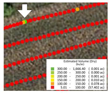
Figure 9: Effects of travel distance error measurement where a quick stop (at arrow) results in a high (1,666 bu/ac) yield data point estimate.
