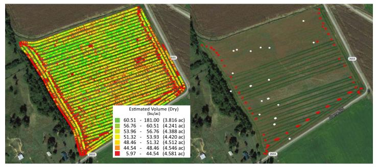
Figure 2: Traditional view of yield map (left) consisting of GPS latitude, longitude, and yield estimate data points. Yield data errors are shown at right, over-estimates (white, >80 bu/ac) generally due to quick deceleration with under-estimates from cut-width, lag time, or header setting errors (red, < 30 bu/ac) around edges of the field.
