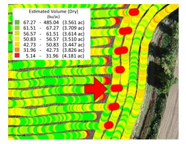
Figure 8: Effects of incorrect lag time settings (and potential GPS offset issue) illustrating data shifted too far along passes.
