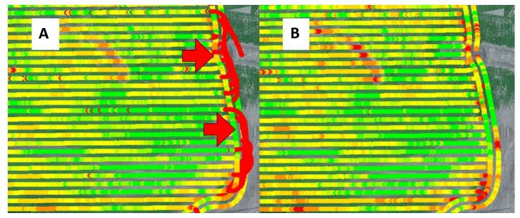
Figure 6: Header position sensor errors in raw yield data (A) and clean yield data after removal of errors (B).
