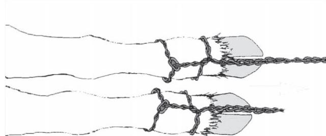
Figure 3. Proper attachment of the pulling chains.
