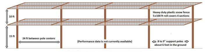
Figure 3. The USMARC high-rise shade design.
