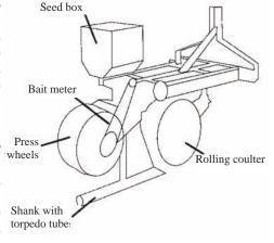
Figure 2. Give basic parts of a burrow builder: 1) rolling coulter, 2) shank with torpedo tube, 3) bait box, 4) bait meter, 5) press wheel(s).
