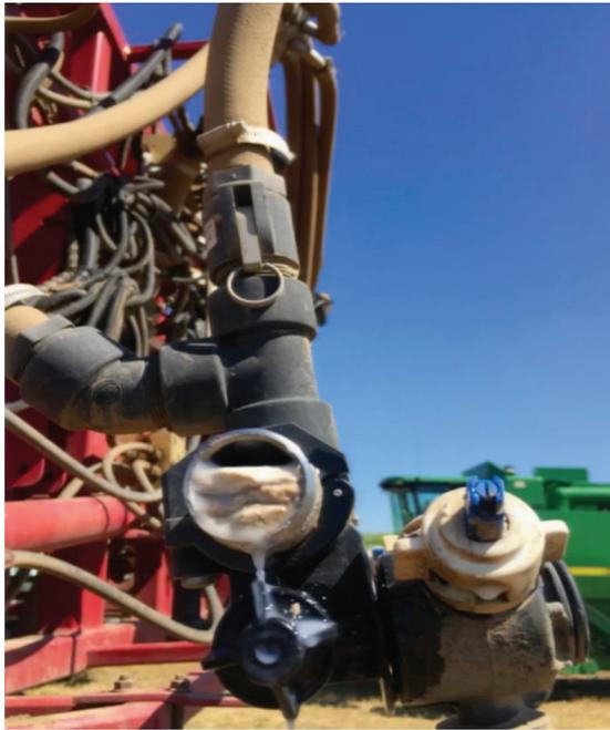
Fig. 2. Pesticide residue accumulation at an end cap.
