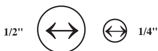
Figure 2. Rats can gain entry through holes as small as 1/2 inch in diameter; mice can use holes as small as 1/4 inch in diameter. (Source: Prevention and Control of Wildlife Damage 1994).
