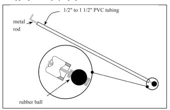
Figure 5. PVC pipe sampler.
