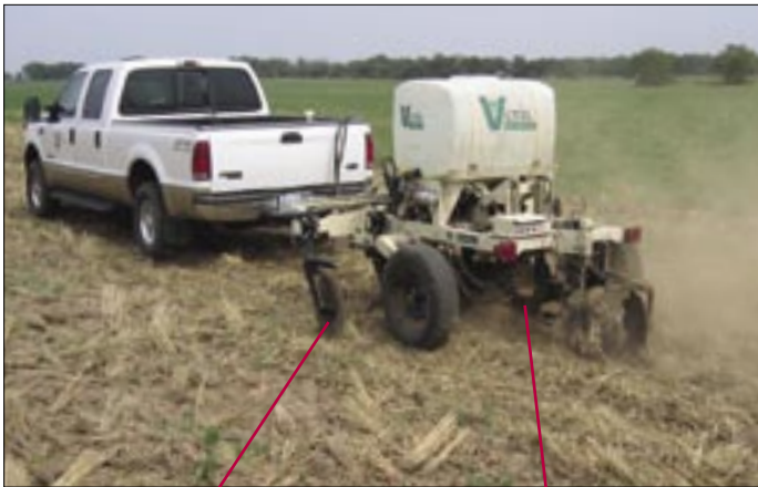
Figure 4. Veris® Mobile Sensor Platform (MSP).
