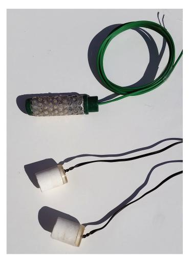
Figure 6. A Watermark Granular Matrix sensor and gypsum blocks.
