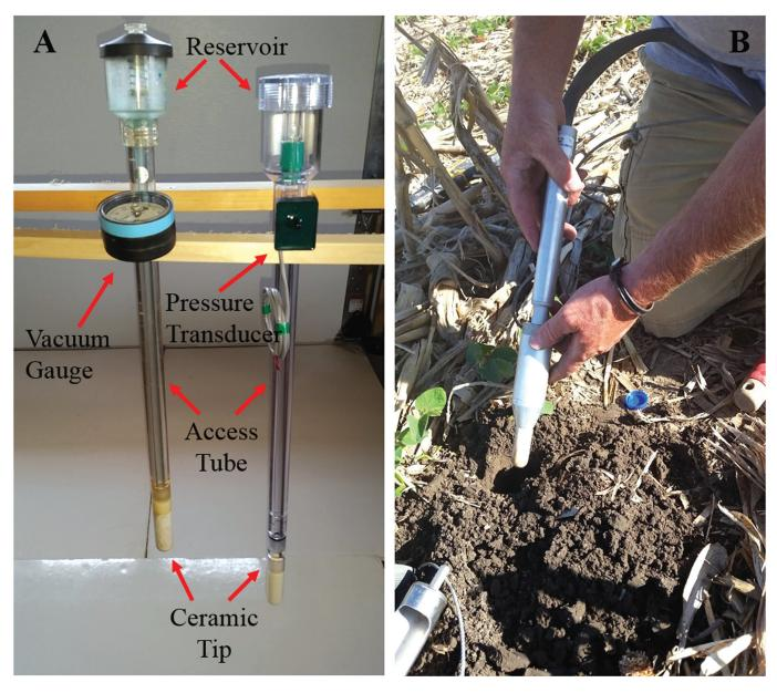
Figure 5. Two traditional tensiometers, one with a vacuum gauge (Soil Moisture Equipment Corp., Santa Barbara, CA) and the second with a pressure transducer (Irrometer Co., Inc., Riverside, CA) (A), and a tensiometer developed by Hortau, San Luis Obispo, CA) (B).
