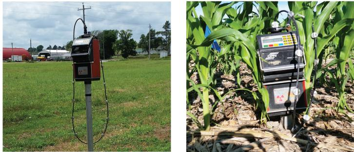
Figure 2. Installation of an access tube (A), standard count measurement (B), and in-season field measurement of a CPN 503DR Hydroprobe<sup>™</sup> (neutron gauge) (C).
