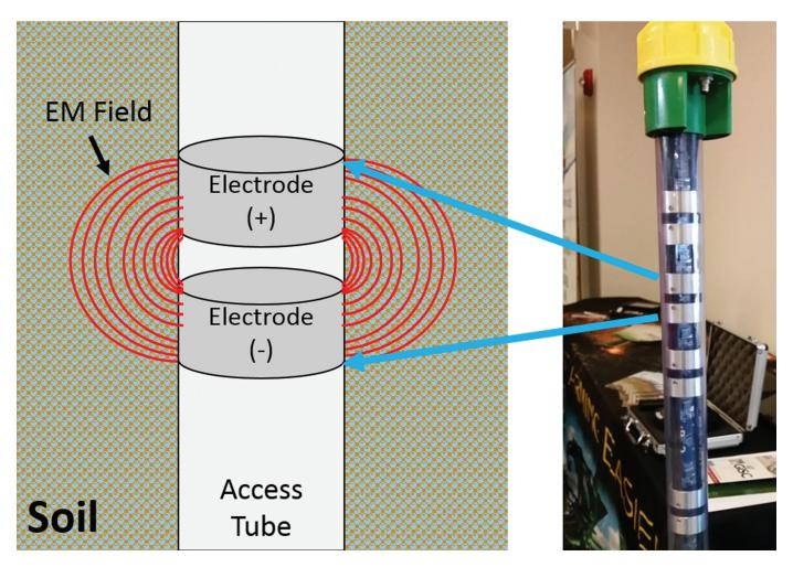
Figure 3. Capacitors located within a John Deere Field Connect<sup>™</sup> capacitance probe with an illustration of a capacitor's electromagnetic (EM) field penetrating the soil.
