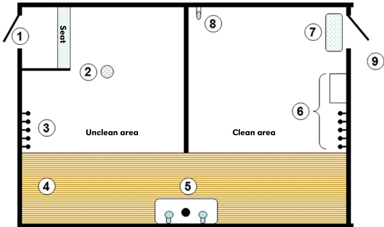
**Figure 4. Danish entry method for a non-shower farm. 1. Only entrance to facility and footwear is removed; 2. Floor drain; 3. Street clothes are removed; 4. Wooden-grate passage is only entered in stocking feet; 5. Hands are washed and disinfected; 6. Protective clothing and boots; 7. Use footbath before entering unit; 8. Water-tap with hose; 9. Pig facility (adapted from Moore, 1992)**
