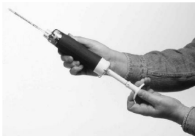
Figure 2. Gas detection pump with a detector tube attached.
