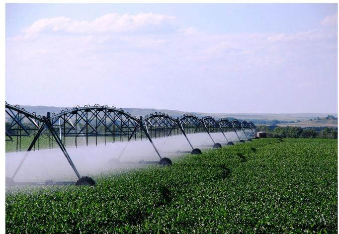
**Figure 2:** A nine-span center pivot system operating in a soybean field in southwestern Nebraska in an early summer morning to assess the uniformity of the water application.
