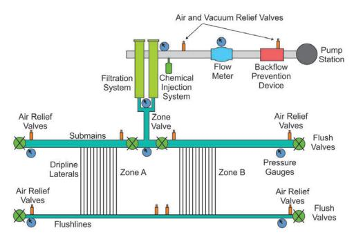
**Figure M-3.** Installation components recommended for an SDI system (modeled after image by Kansas State University).
