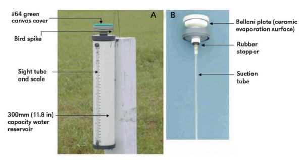
Figure I-8. ETgage used to estimate reference crop ET.
