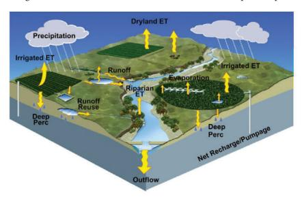
Figure H-5. Diagram of the major water balance components of a typical agricultural watershed.
