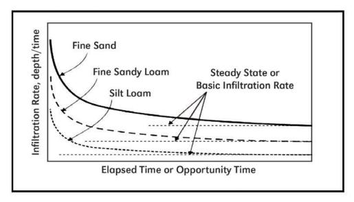
**Figure C-7.** Infiltration rate vs. infiltration opportunity time graph for a fine sand, fine sandy loam, and silt loam soil.
