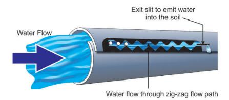
Figure M-2. Schematic drawing of a subsurface drip emitter.
