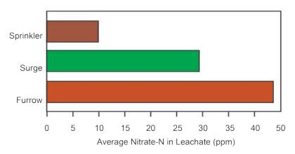
**Figure A-5.** Average nitrate-nitrogen concentrations in leachate water below corn fields irrigated by sprinkler, surge flow, and traditional furrow irrigated fields in the Platte Valley. (See Spalding, et al., 2001).
