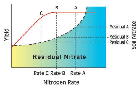
Figure G-3. Impact of excessive nitrogen application rate on soil residual nitrogen.
