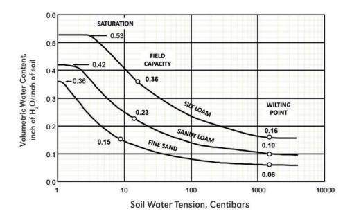
Figure C-6. Soil water retention curves for three soil textures.
