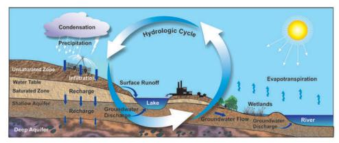
Figure H-3. Diagram of the hydrologic cycle (source www.sws.uiuc.edu/docs/watercycle).
