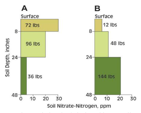
**Figure D-9.** Summary of two sets of soil samples: A) taken from soil that was sprinkler irrigated; and B) taken from soil that was irrigated by a furrow irrigation system.
