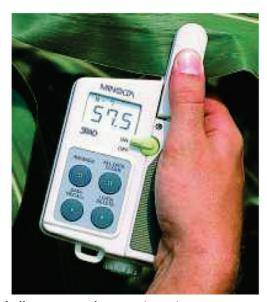
Figure G-6. Handheld chlorophyll meter used to monitor nitrogen status of corn plants.
