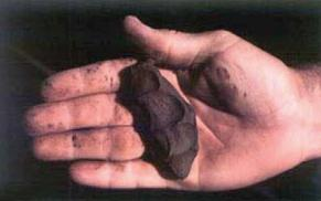
Figure J-3. Sampling and evaluation techniques for the feel method of soil water monitoring.
