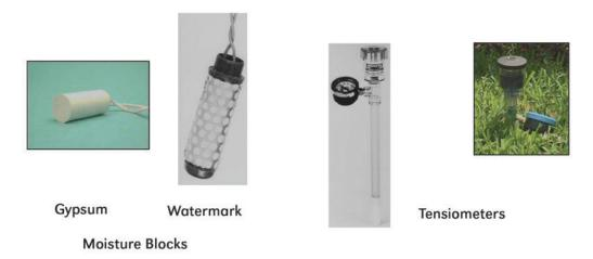
Figure J-4. Methods of measuring the soil matric potential.
