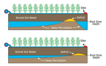
**Figure K-3.** Infiltration profiles under conventional furrow irrigation with blocked-end furrows (top) and three-quarter-plus advance rule (bottom).
