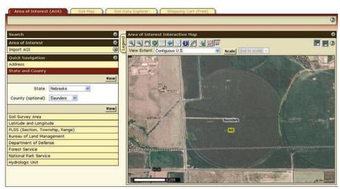
**Figure J-10.** Web Soil Survey webpage used to obtain soil mapping units, field slopes, and soil properties useful when scheduling irrigation events and for designing irrigation systems.
