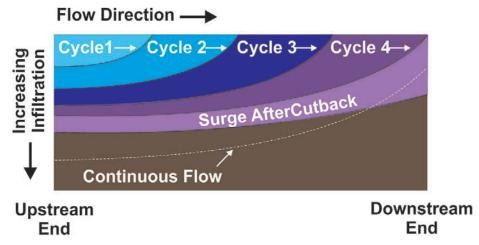
Figure K-7. Comparison of infiltration profiles for surge and continuous flow furrow irrigation systems.
