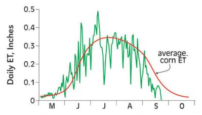
**Figure I-5.** Comparison of the long-term average ET rate for well-watered corn and the daily ET for a specific year.
