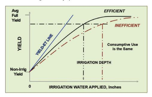
Figure H-9. Effect of improved irrigation efficiency on in-field water use and yield.
