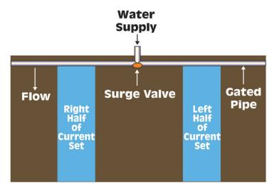
Figure K-6. Typical surge irrigation field layout.
