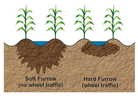
Figure K-8. Differences in water infiltration patterns under non-wheel track and wheel track furrows.
