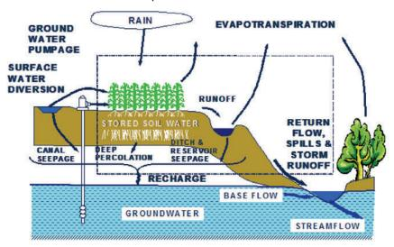
**Figure H-7.** Diagram of water balance for an irrigated field supplied with ground and surface water for irrigation.
