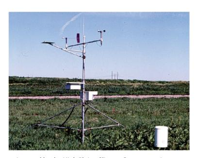
Figure I-7. Weather station used by the High Plains Climate Center to estimate crop water use.
