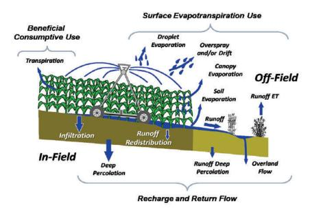
Figure H-8. Water balance components for irrigated cropland.
