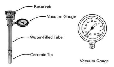
Figure J-5. Components of tensiometers used to measure soil matric potential.
