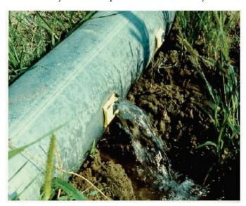
Figure K-1. Typical gated pipe furrow irrigation system.
