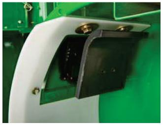
Figure 1. Impact plate mass flow sensor located at the top of the clean grain elevator.
