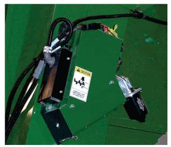
Figure 5. Moisture sensor located on the side of the clean grain elevator.
