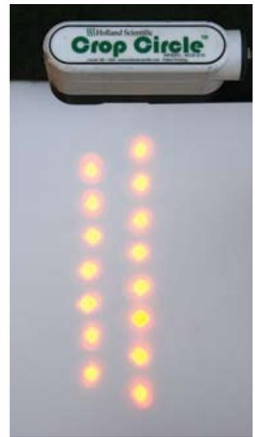
Figure 5. Crop canopy sensor (Crop Circle, Holland Scientific) illustrating the emitted light pattern.
